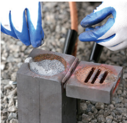
4. Sprinkle the starting powder over the weld powder and onto the lip of the mold. Close the cover.
