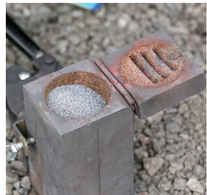
3. Dump weld powder into crucible.
