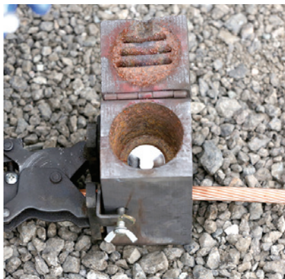
2. Place metal disc in bottom of mold crucible.
